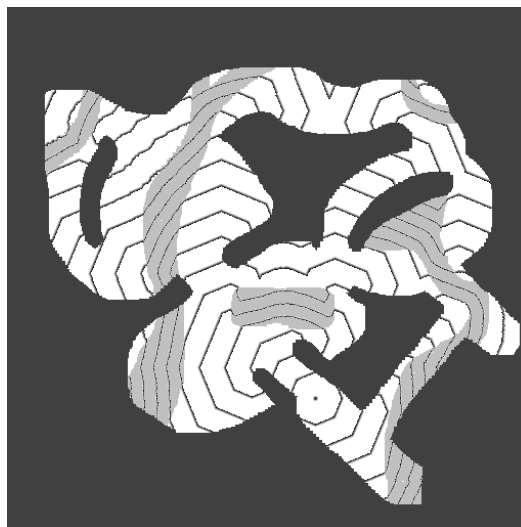
Fig. 1. An example of a distance map with a weighting of \gamma = 1 , so that paths through lava have twice the weight of paths through empty space. The contour lines correspond to distances a multiple of 25 pixels from the origin (shown as a dot). Note that in regions of lava (shaded light grey) the contour lines are closer together.
